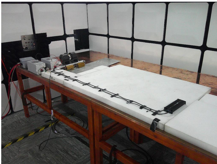
Photo 2.2-1 – RE102 General Setup
