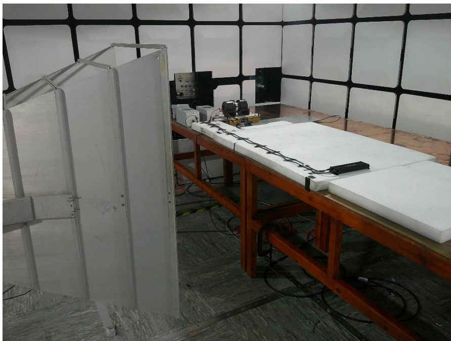
Photo 2.2-7 – RE102 Test Setup – 200 MHz – 1 GHz
