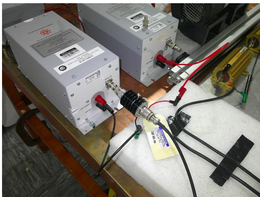
Photo 2.1-6 – CE102 Test Setup – LISN 2 (DC-)
