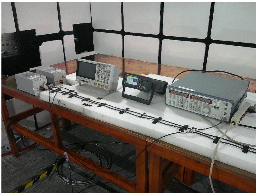
Photo 2.1-3 – CE102 System Check Setup
