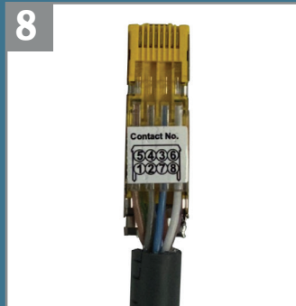
8 Picture of completed First Assembly of cable.
