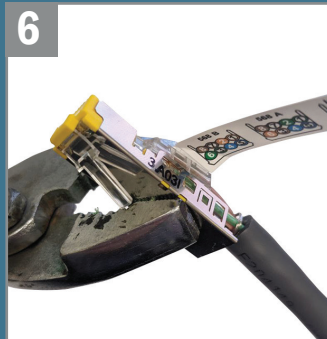
6 Clamp wire guide down onto contacts as shown.
